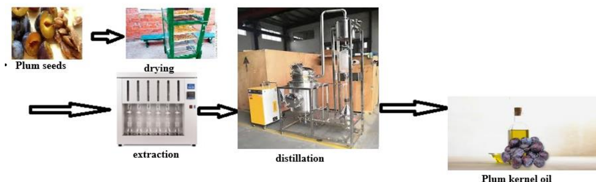
Figure 1. Extraction technology of plum oil.
